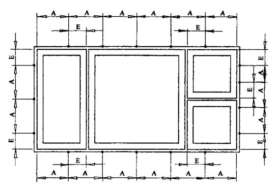
A < 700 mm; E = 150 mm; For laminated PVC E = 250 MM.
